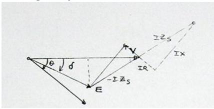
For a lagging pf,  $E\angle -\delta = V\angle 0 - I\angle -\theta * Z_s \angle \beta$
