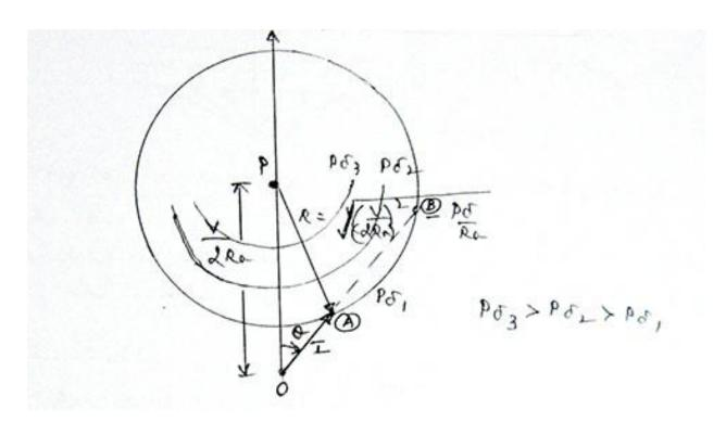
The above equation shows the locus of current for constant P $\delta$  is a circle with radius  $((V/4R_a^2)-(P\delta/R_a))^{1/2}$  with centre at  $(V/2R_a)$  from the origin 'O'.
