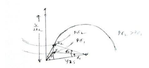
When the load is increased suddenly, the rotor momentarily reduced in speed increasing the value of load angle to ' $\delta_2$ ' from ' $\delta_1$ ' to develop more power to meet the increase in load. But it does not stop exactly at the required new value ' $\delta_2$ ' but slightly over shoots developing more power than required.
