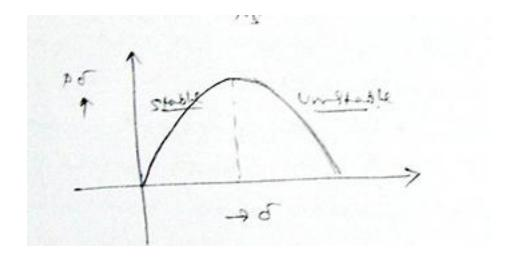
Salient pole synchronous motors are more stable than wound rotor motors due to interlocking of DC poles with rotating magnetic flux.
