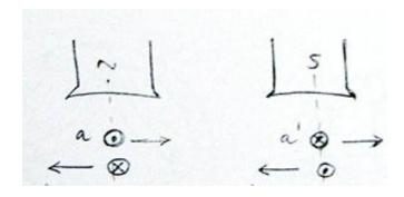
When conductors **a** and **a**' are under N pole and S pole respectively, the torque produced is in a direction to move the conductors from left to right. But, since the input applied to the conductors **a** & **a**' is ac, within half-a-cycle the current in '**a**' changes to 'cross' and the current in '**a**' changes to 'dot' making the conductors to move from right to left as shown in the fig.
